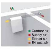
Expandable for even more flexibility. Adjoining rooms can also be integrated into the ventilation system as a result of the adjoining room connection. Large residential units can use several units to supply and extract air.
