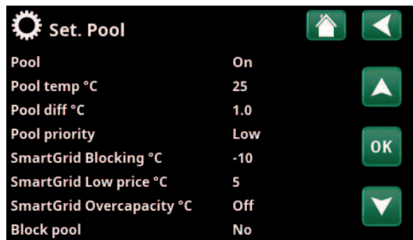
Menu: "Installer/Settings/Pool". The pool temperature is increased by 5 °C when the SmartGrid Low Price function is activated.
